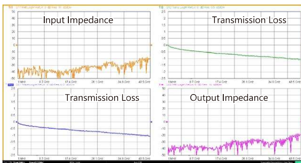
Measurement of input/output impedance and transmission loss, Characteristic impedance evaluation (TDR)
