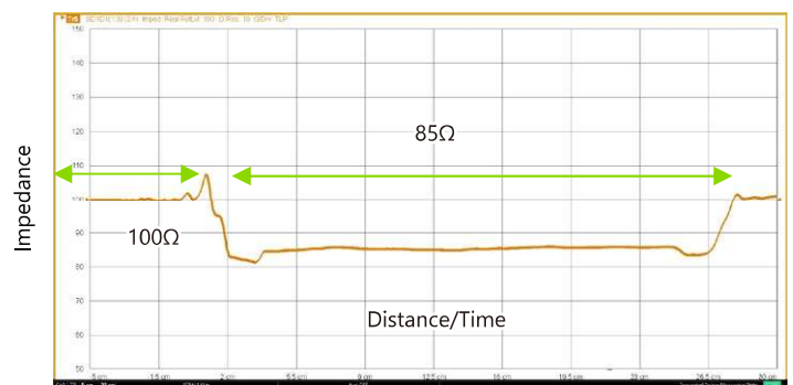
Characteristic impedance evaluation (TDR)
