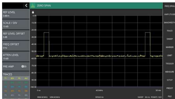
TPMS pulse measurement (zero span)
