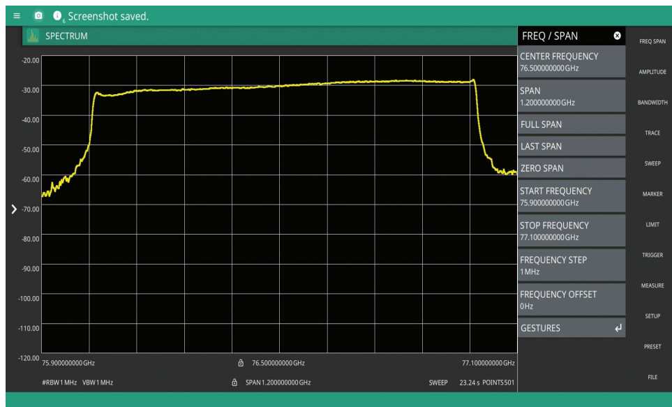
Figure 3. The Spectrum Master MS276xA Captures the Envelope of Automotive Radar FMCW Chirps from an Over-the-Air Measurement
