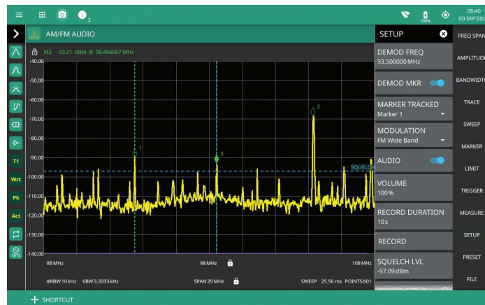
AM/FM Signal Demodulation at Marker Frequency
