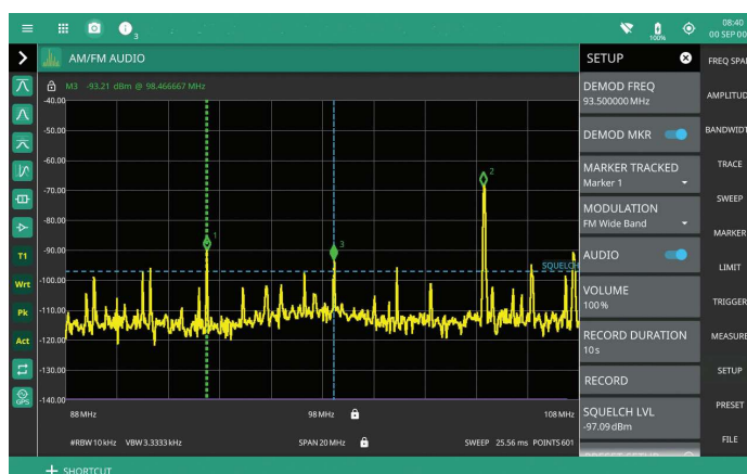
AM/FM Signal Demodulation at Marker Frequency
