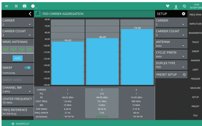
Use Carrier Aggregation Mode for Over-the-Air (OTA) Capture of Multiple LTE Signals
